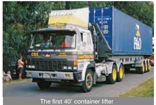
The first 40' container lifter
