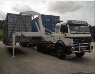
The High Lift has the ability to load and unload a container from an adjacent trailer while the Swinglift is itself loaded with a container.
