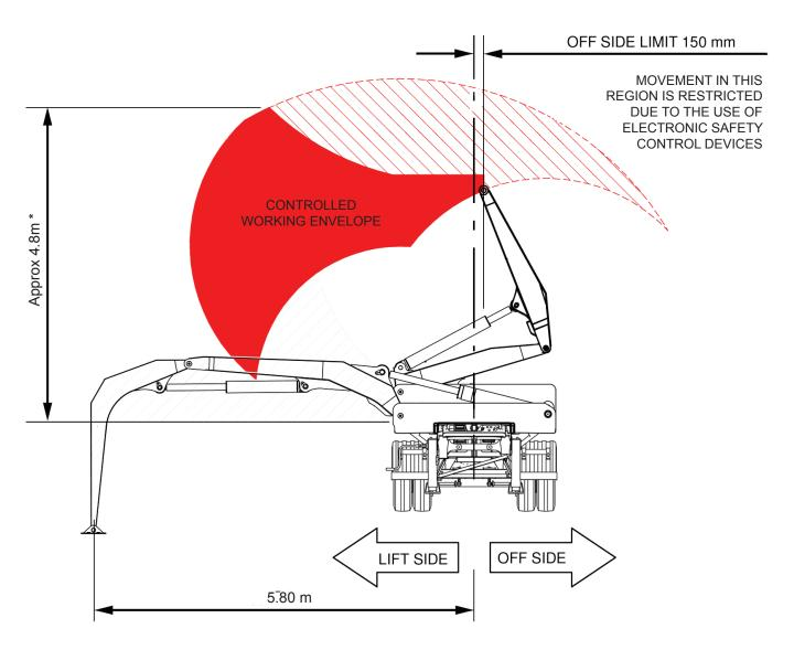
\* Dimensions may vary depending on trailer running equipment i.e. axles, wheels and suspension required in country of destination.
